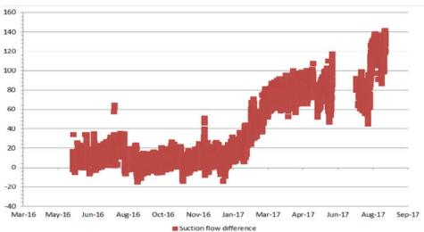
To diagnose the anomaly, the team tested suction flows using a portable ultrasonic flowmeter. Vibration data was recorded at regular intervals. They also checked the recirculation valves in the boiler feed water pumps and looked for clogs in the suction strainer. After performing these tests, in conjunction with continuous performance monitoring, they determined that the pump had a mechanical (internal) issue. The team also identified a faulty suction valve.
